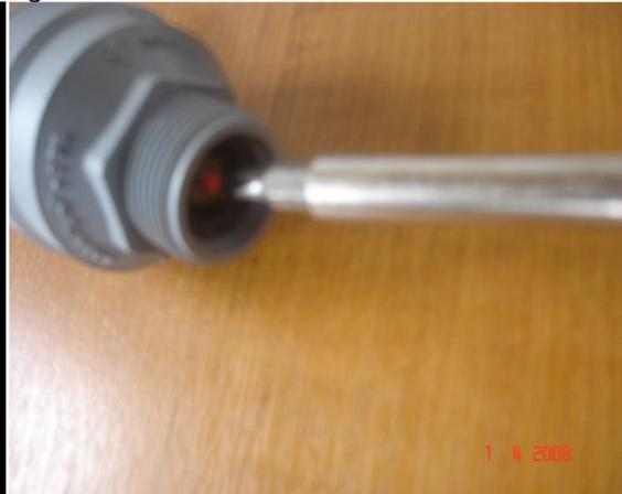
On then end that was connected to the pipe you will see a little red button Fig 7 . Press the button hard with a pen or small screw driver Fig 8 and you may get a small amount of water coming out. Press it again for good measure and reconnect.
