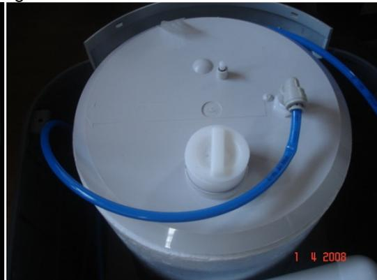
Once the lid is off there is a small round tank lid FIG 2 with a blue pipe feeding into the top. There may be a small white button on the lid which can be pushed to resetting the floats below Fig 3 . Sometimes this needs pressing a couple of times. If there is no little white button on the lid gently ease the tank lid off Fig 4 and you will see the floats on the under side. Gently move the floats up and down if removing the lid has not already caused the water to flow.
